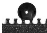
Water droplets on the surface of an aluminum alloy with a T-shaped microstructure
