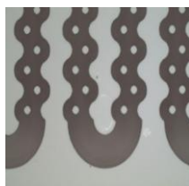
optical microscopy image of the gas chromatography column
